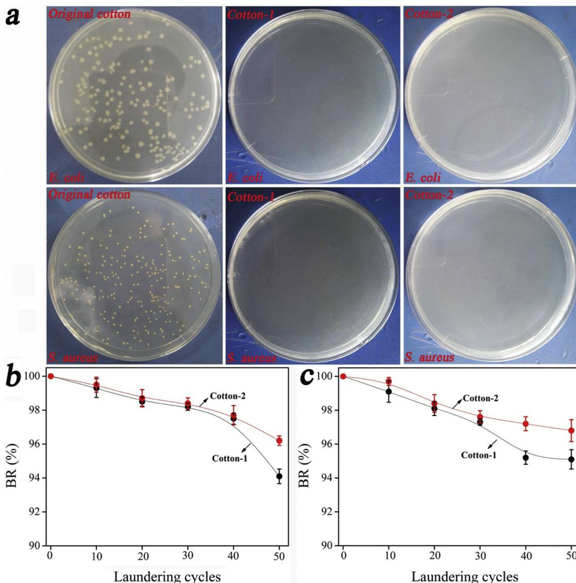
Fig. 6. The antibacterial effect of the cotton fabric samples, the optical images of the antibacterial tests (a), and the durability results of the antibacterial properties against *E. coli* (b) and *S. aureus* (c).
