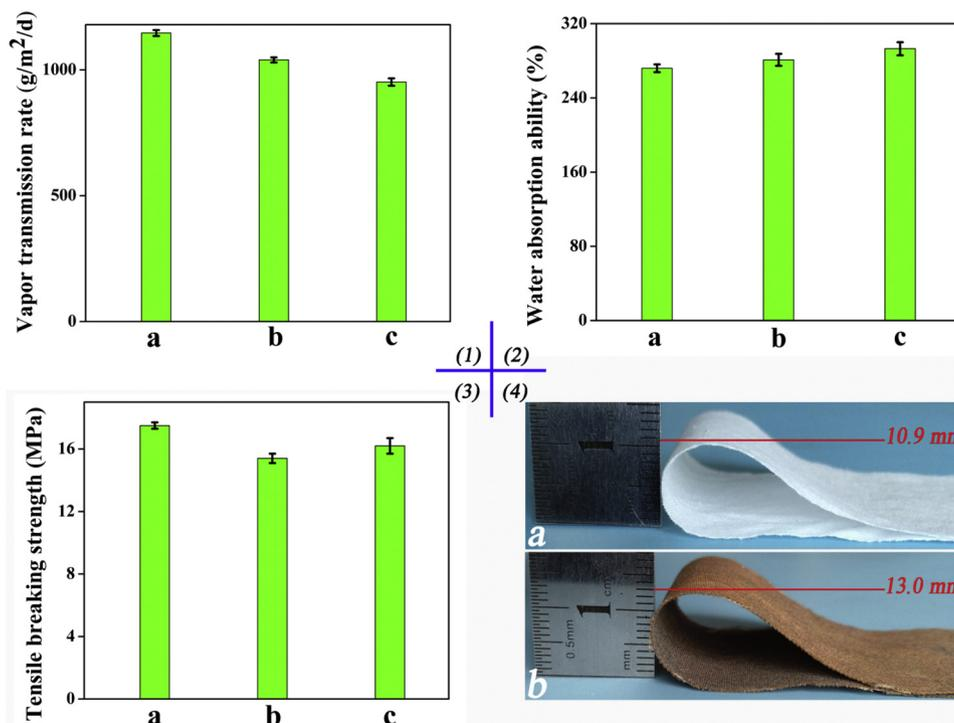
Fig. 8. Influence of the surface modification on the nature of cotton, including (1) water vapor transmissibility, (2) water absorbability, (3) tensile strength, and (4) flexibility. (a) Original cotton, (b) Cotton-1, and (c) Cotton-2 fabric samples.
